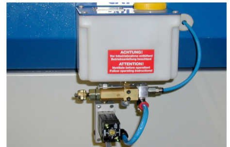
Minimalmengen-Schmierung optionale Systeme Minimum quantity lubrication optional systems
